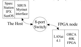
**Figure 4: Performance test configuration**
